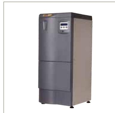
The Parker domnick hunter zero nitrogen generators employ robust, field proven technology to produce ultra high purity nitrogen for GC makeup and carrier gas applications. An integral heated platinum catalyst ensures carrier grade nitrogen free from organic impurities to <math><0.1\text{ ppm}</math>.
